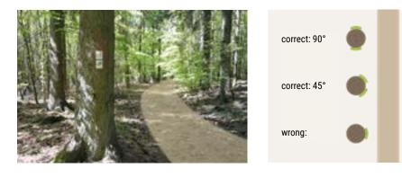
**2.** Waymarks must be placed equally for both directions of travel. On longer stretches, they should preferably be on the same side of the path. Care must be taken to ensure good visibility and easy maintenance.
