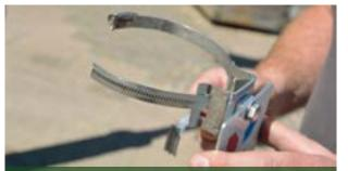
Variant a: with hose clamp and U-shaped holder (size of the band can be adjusted)
